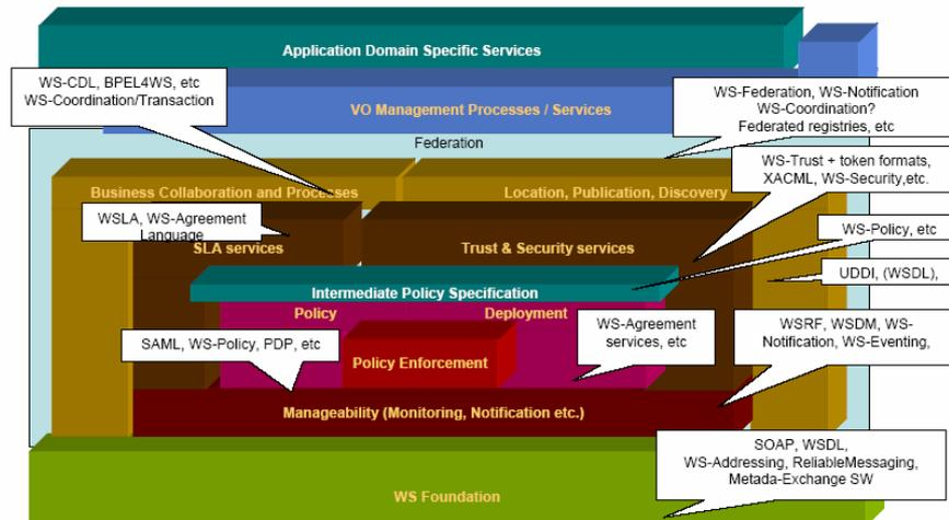
Figure: A component architecture to support the TrustCoM framework for security, trust and contract management of dynamic VO.
