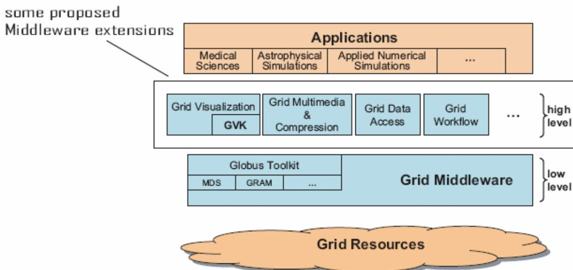
Figure: The Architecture of the Austrian Grid incorporating the GVK.
