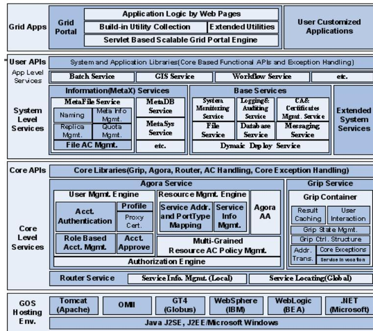
Figure: CNGrid Grid Operating System (GOS) Architecture
